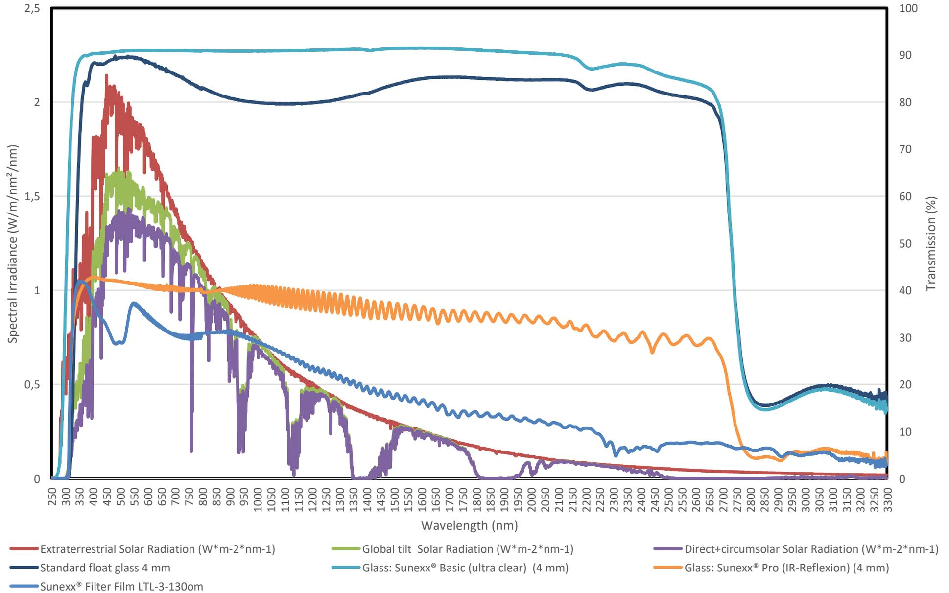
ASTM G173-03 Reference Spectra derived from SMARS v 2.9.2 - Measure of Transmission by Varian Cary 500 Spectrophotometer
